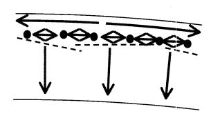
**Concrete Shrinkage and Failure Planes**
